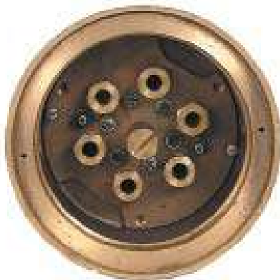
ELECTRICAL COMPARTMENT (Dry upper chamber)
